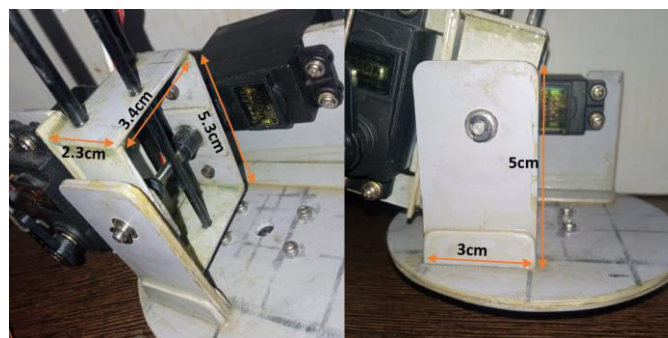
Fig 8. Lower Joint Box
