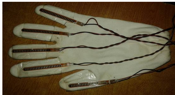
Fig.7: Hand gloves using flex sensor [15]
