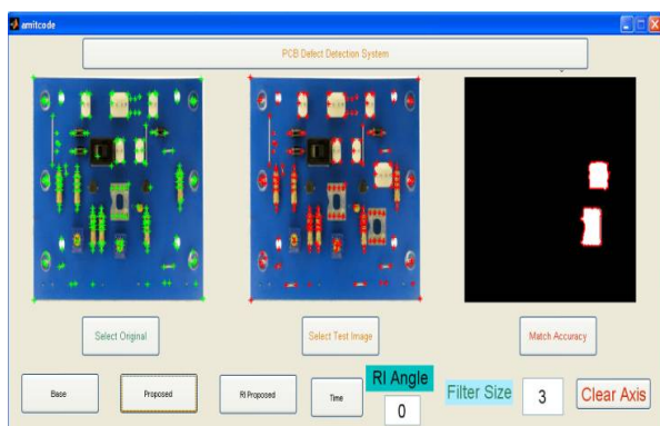
Figure 10- Result of proposed system on component placed PCB
