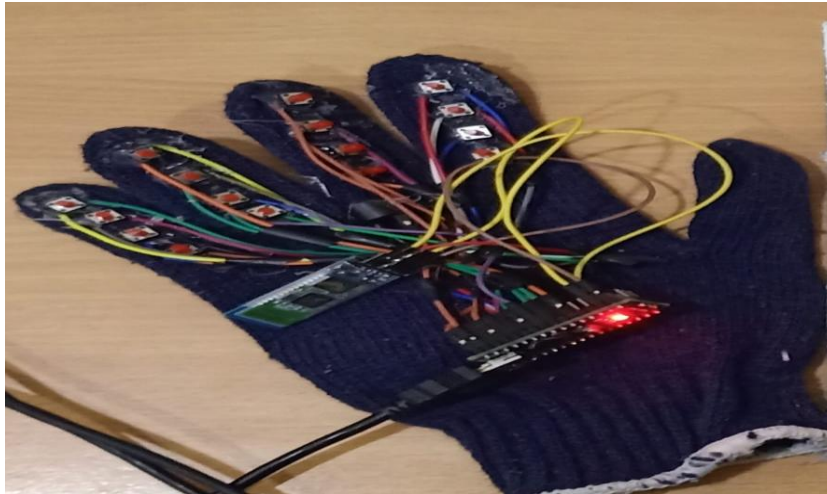
Fig 5.1 Glove Fitted with Buttons and Arduino
