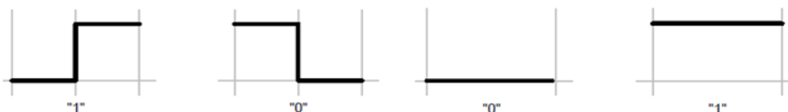
Figure 5: CAN Bit encoding (a) Manchester encoding (b) NRZ encoding
