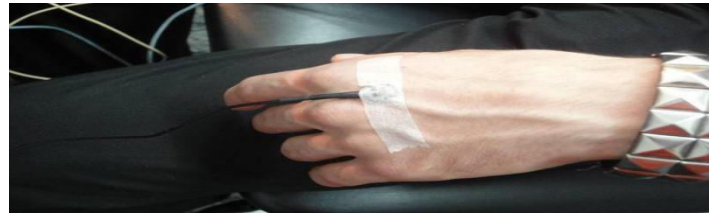
Figure 4.1 Example of reference disk electrode placement
