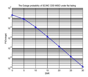
Fig. 2. The Outage probability of SC/MC CDD MISO under flat fading with three transmit antennas and R = 2 b/s/Hz.
