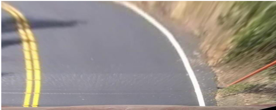
Fig.4: Frontal to top view perspective transformation
