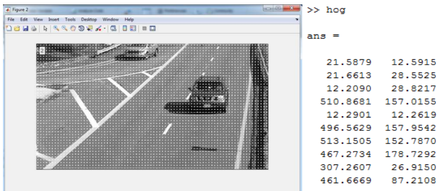
Figure 4: HoG feature points are extracted from the video frame and the required ten strongest HoG points are extracted marked and displayed as the output.
