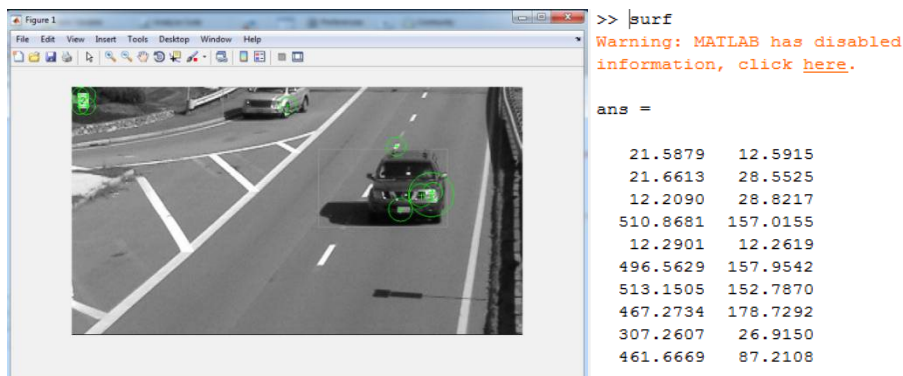
Figure 1: SURF feature points are extracted from the video frame and the required ten strongest SURF points are extracted marked and displayed as the output.
