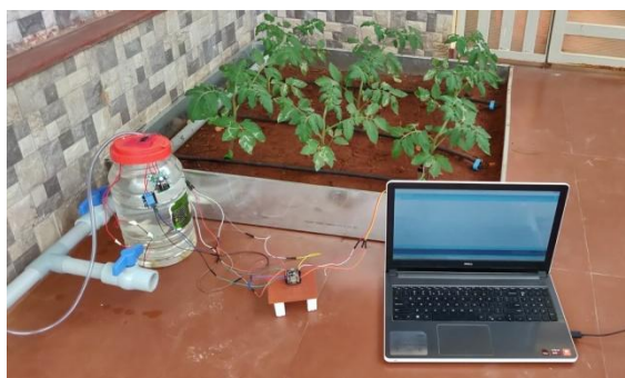
Figure 5: Hardware setup of drip irrigation system.
