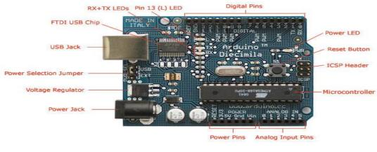
Photograph by SparkFun Electronics. Used under the Creative Commons Attribution Share-Alike 3.0 license Figure 1: Arduino Circuit
