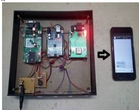
Fig.6 Working Structure of Accident Detection and Intimation using GPS and GSM
