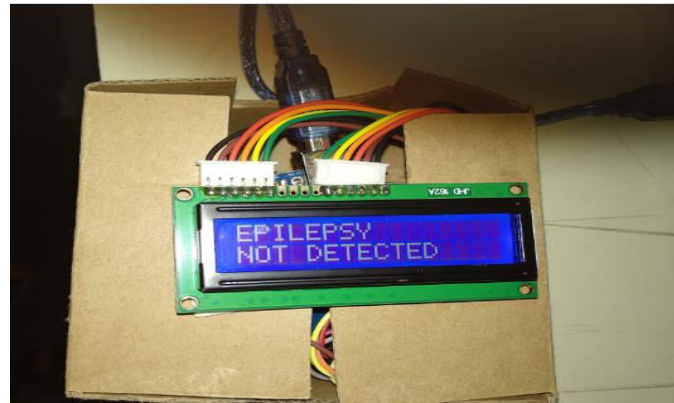
Figure. 4.10: Output of LCD showing result “EPILEPSY NOT DETECTED”
