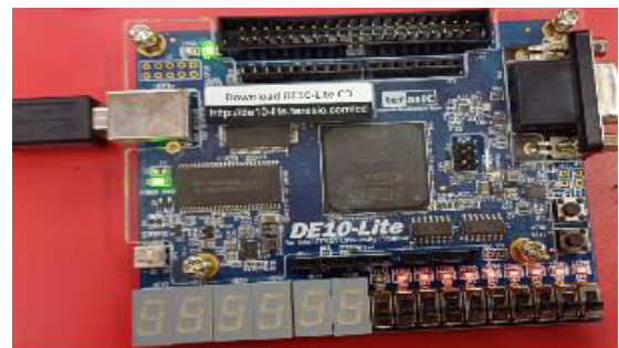
Fig. 11. Implementation on DE 10 LITE INTEL FPGA
