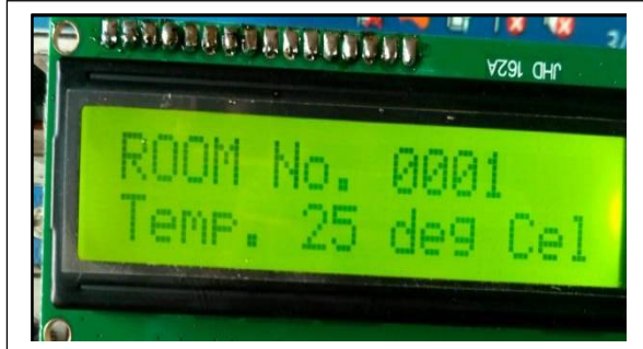
Fig.8: LCD shows temperature status of room no.1
