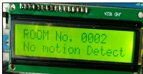
Fig.11: LCD shows motion status of room no.2
