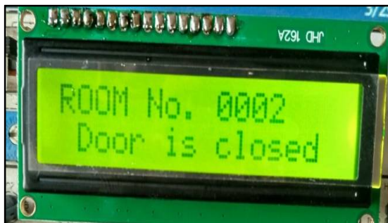
Fig.10: LCD shows door status of room no.2
