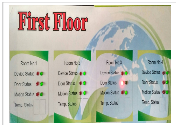
Fig.13 Display panel shows door of room no.3 is opened.
