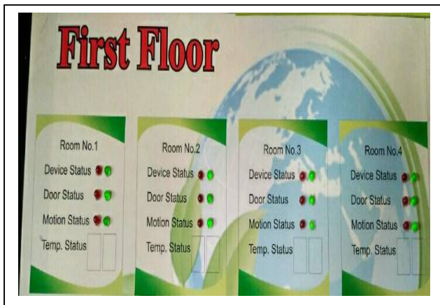
Fig.12 Display panel shows normal status of all the rooms
