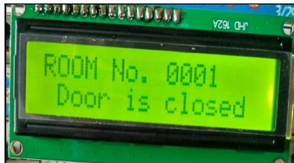
Fig.9: LCD shows door status of room no.1
