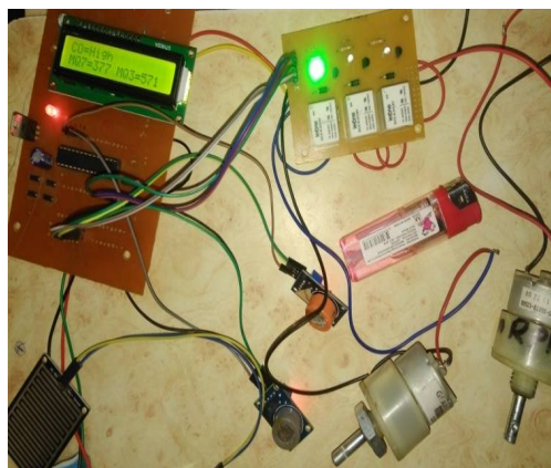
Fig. a) Output of CO Sensor goes high
