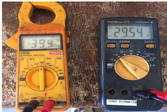
Figure 11: Input voltage and Output voltage
