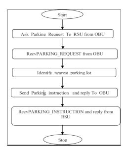
Following steps shows the communication between the OBU to OBU, and OBU to RSU and vice versa. 1. Ask Parking Request To RSU from OBU:
