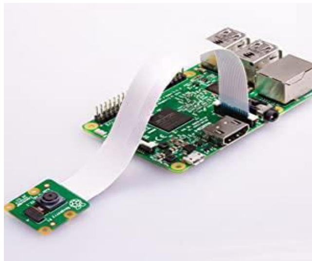
Figure 5: Pi Camera interfaced with Raspberry Pi for Facial Recognition and Traffic Light Detection.
