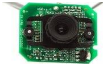
Fig. 3. Integrated webcam and microphone circuit board
