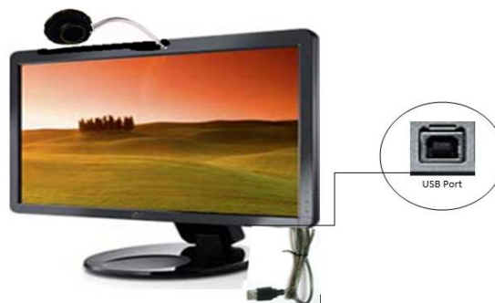
Fig. 4. Proposed prototype of LCD monitor with flexible built-in Webcam and Microphone
