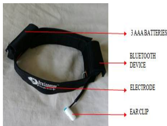
Fig.2. Photograph of our wireless brain wave sensor with an electrode, a Bluetooth, batteries and an ear clip.
