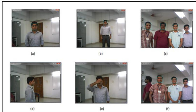
Fig. 10.(a) The target is in close proximity about 2meters, (b) The target is away about 4meters, (c) Four targets appears simultaneously on the screen, (d) The target turns 90 degrees, (e) Target hides its eyes, (f) Three targets face towards the camera and one is at 90 degree
