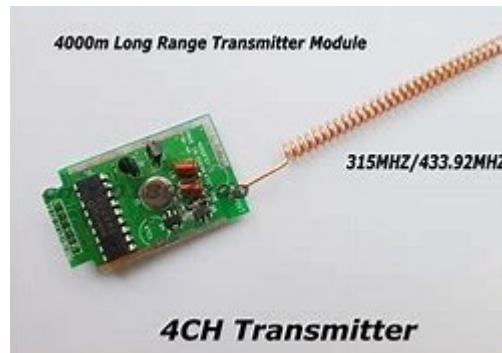
FIG 5.1: DETAILED VIEW OF WIRELESS TRANSMITTER
