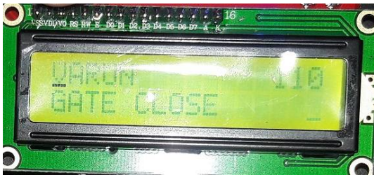
Figure 10: LCD Display gate close message to stepper motor
