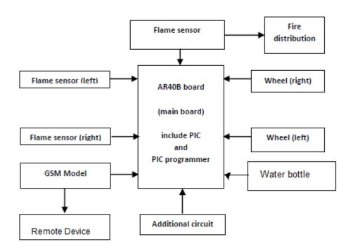
Figure shows, System Architecture of fire fighting robot with GSM using Microcontroller. It consists eleven blocks. Basically system architecture of fire fighting robot is divided into three main parts:
