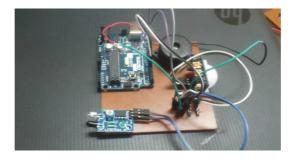
As shown in above figure, it is an indoor unit it consists of PIR sensor, IR sensor it counts the number of intruders enter into room or stores, it consists ultrasonic sound replier itgives sound to avoid the animals and it consists temperature sensor it maintains the room temperature this outdoor unit focuses on secure the warehouse management from thief and animal detection, monitor of the room temperature.
