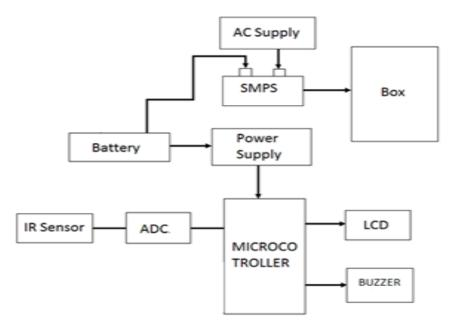
Fig1: Block Diagram of Smart Refrigeration System
