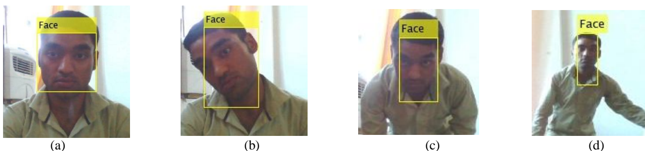
Fig: 2 (a) Detected face with no error (b) Detected face with tilt error(c) error while moving backward (d) error while tilting at some distance.
