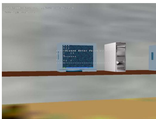
Fig.1. Snapshot of a proof-of-concept 3-D virtual environment, where the user is typing a textual password on a virtual computer as a part of the user's 3-D password.
