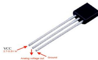
Figure 3: LM35 temperature sensor
