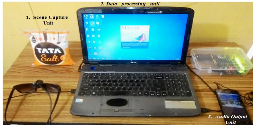
Fig.8 System overview with its three function
