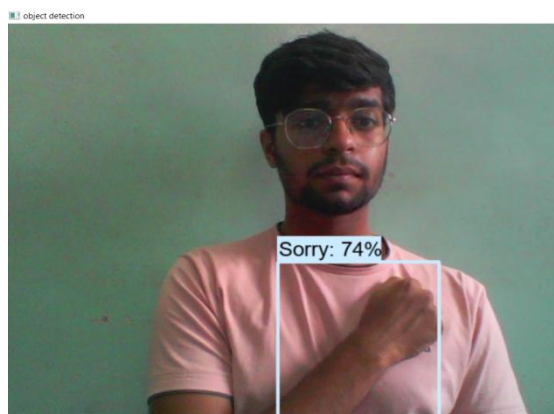
Fig 3: “Sorry” sign detected in real time by the software.
