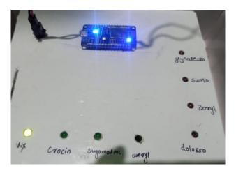
This is an android application at low cost, useful model for an automatic medicine box detector using simple electronics applications. For easy detection and alert, LED has been attached so that the person in medical lab is concerned and can give the right medicine to his customer in time and the right quantity without personalized supervision. This easy way to use device can be a convenient option for all medical stores.
