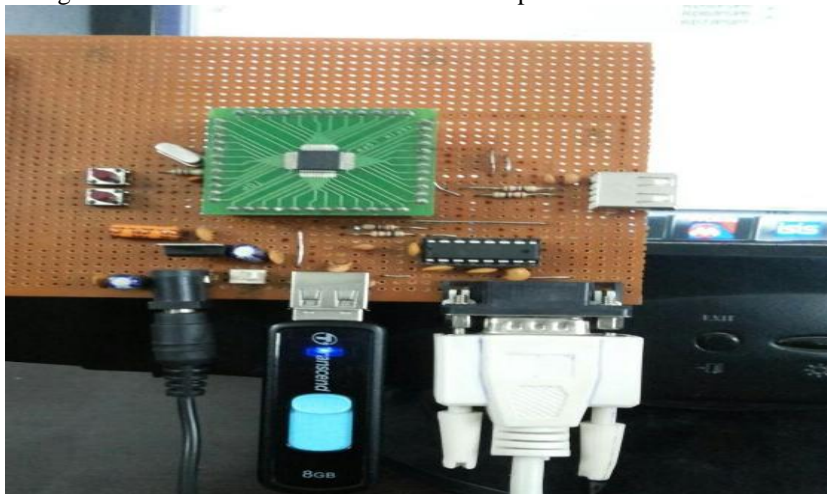
Fig. 3.VNCIL serial interface to PC via RS232 and Hyper Terminal
