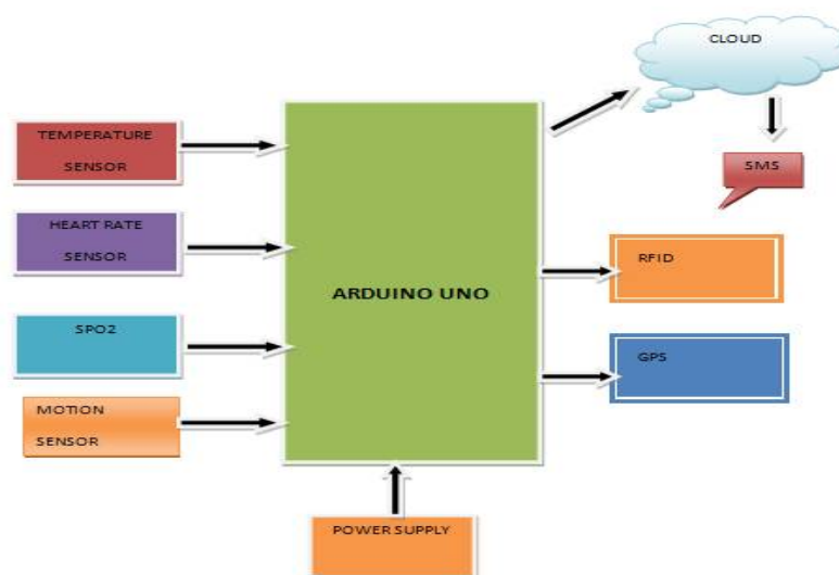
Figure.3: Block diagram of Health monitoring system
