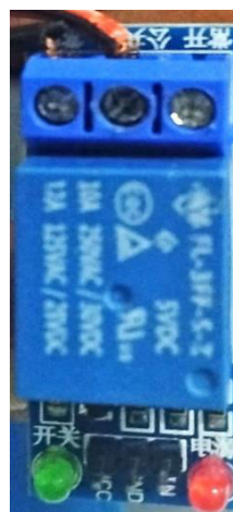
Figure 5.2.2 Power Relay Module
