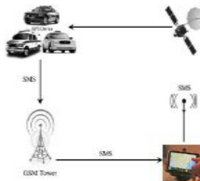
Fig. 1: The block diagram of GPS tracking system
