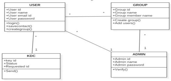
This system diagram is all about various modules that present in system this are shown by various classes which contain the combination of attributes and behaviour that performs various operation related to the classes. How that classese are connected to each other that all are shown in this system design.
