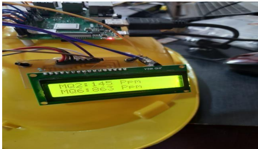
Fig7. Air quality sensor output
