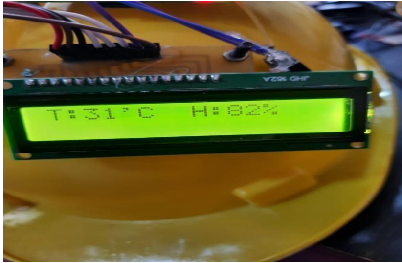
Fig 6. Temperature and humidity output
