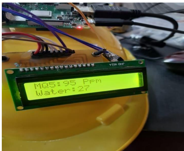
Fig5. Water and gas sensors output
