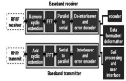
FIGURE 2: A high-level block diagram of the tranceiver baseband processing section in a 4G wireless design
