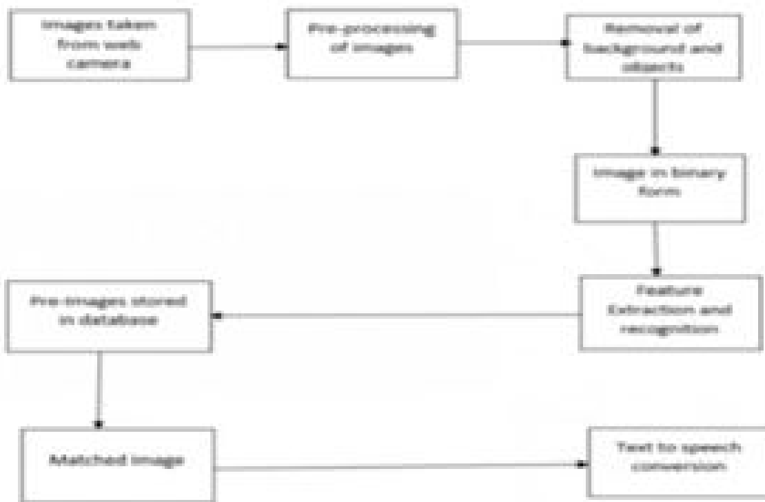
Fig (1.2) System Architecture
