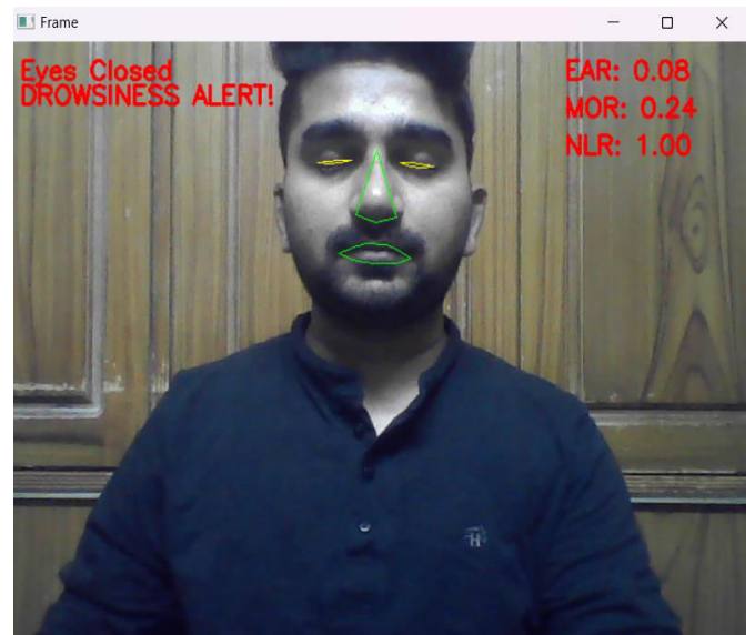
Fig.4 Drowsiness detected by the system due to eye closing
