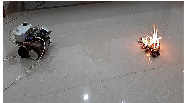
Fig.7. Fire Fighting Robot near the Fire
