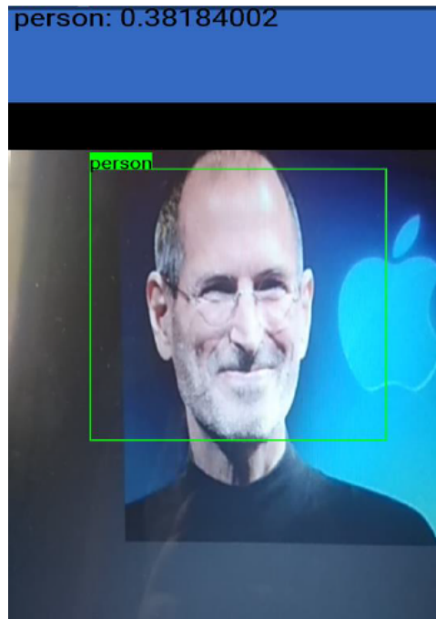
Fig 2. The smartphone has detected 'person' is in the view of camera.
