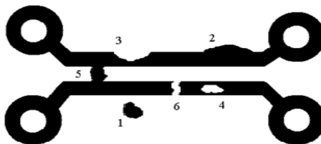
Fig. 1 - Example of a PCB layout defects:
