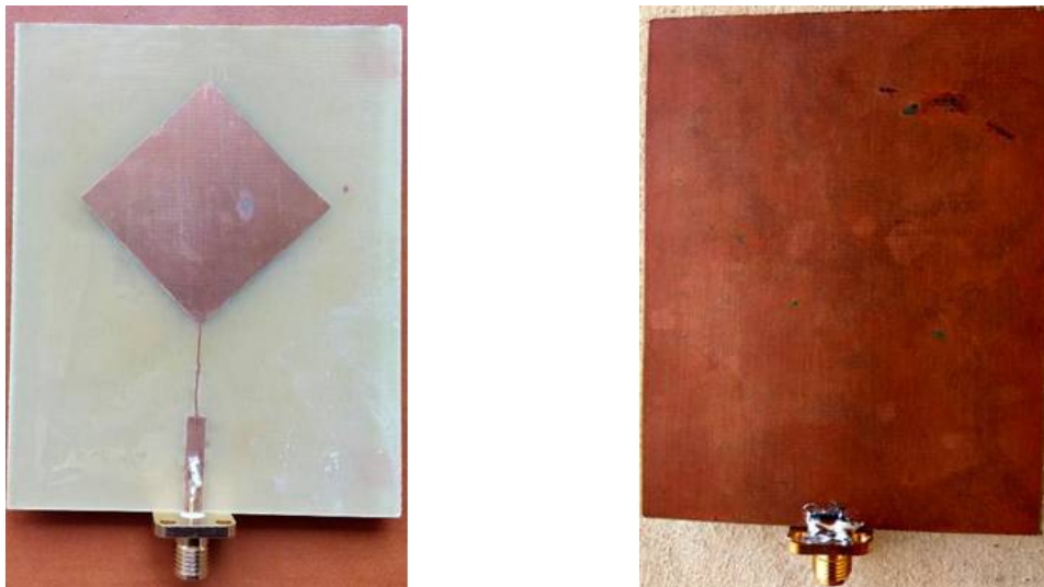
Fig 4: Rhombus shaped microstrip antenna with microstrip line feeding top and bottom view
