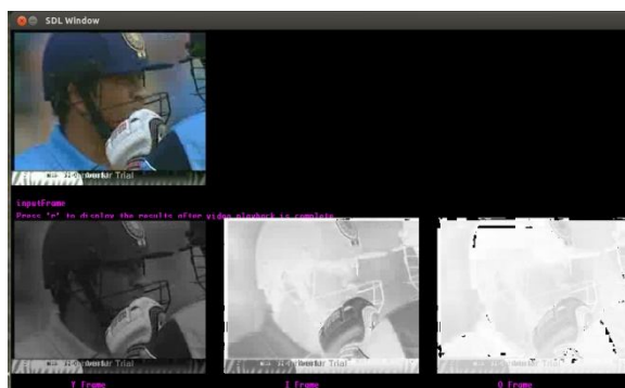
Fig 14 Output of Histogram difference method using YIQ color model
