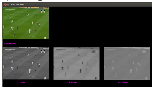
Fig 7 Output of Pixel difference method using YCbCr color model
