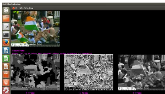
Fig 12 Output of Pixel difference method using HSV color model
