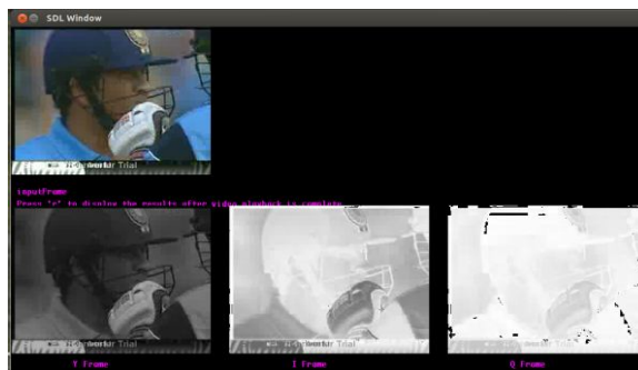
Fig 8 Output of Pixel difference method using YIQ color model
