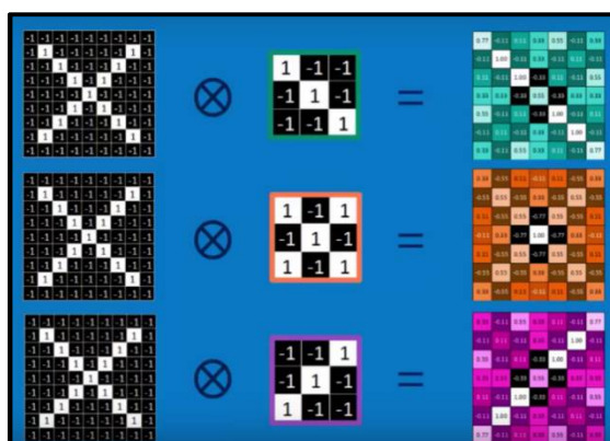
Fig. 3: Convolving each filter with all image matrices to obtain various feature maps
