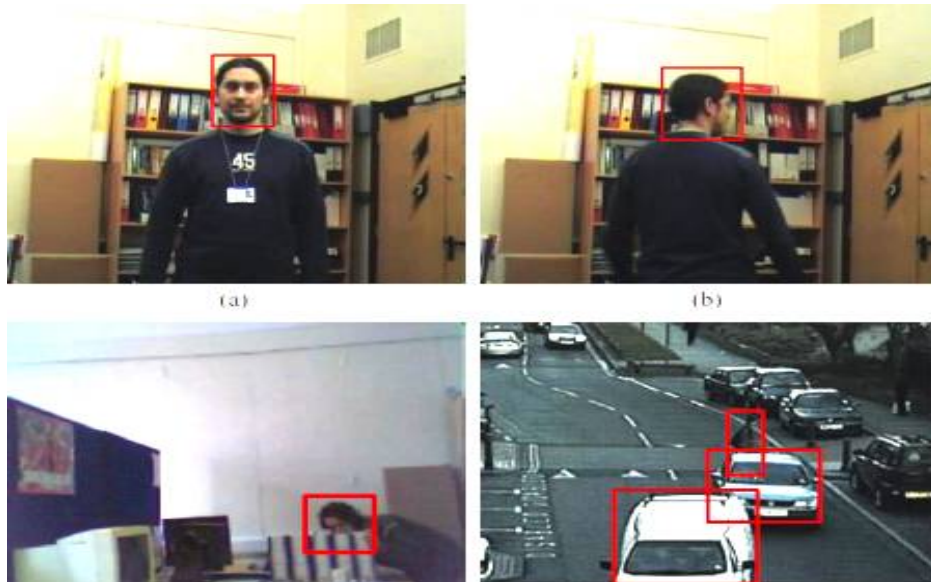
Fig. 1: shows particular appearance that make object tracking difficult. (a)– (b) A reference point to shoot at head changes its pose then its appeared. next: 2 examples are target of occlusions. (c) referenced /referred is hide by still things in the scene. (d) The particular shoot the object is occluded by another moving substances in picture.
