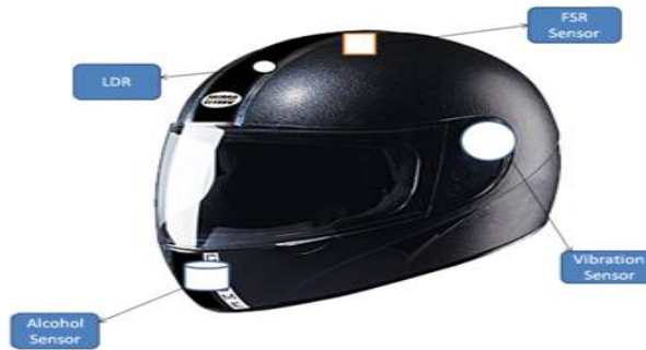
Fig 4. Conceptual Diagram of Helmet with Different Sensors
